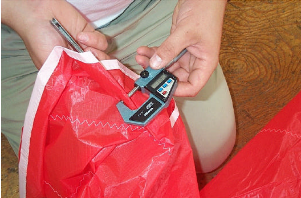
Figure 2. Measuring the thickness of Ply
